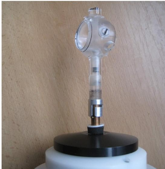
3. Continue pressing the holder downward until you overcome the pressure of an elastic pad under the shank of the holder.
