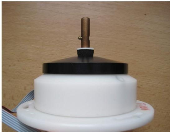
2. Turn the holder until the drive pin enter the notch of the holder:
